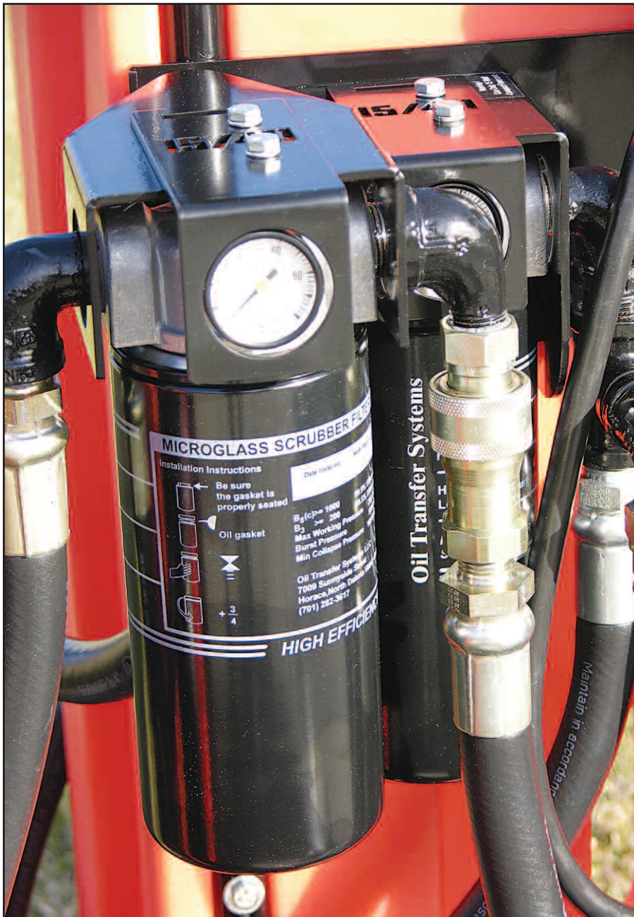
Oil Transfer Systems filter unit includes a gauge and quick-connect hoses.
