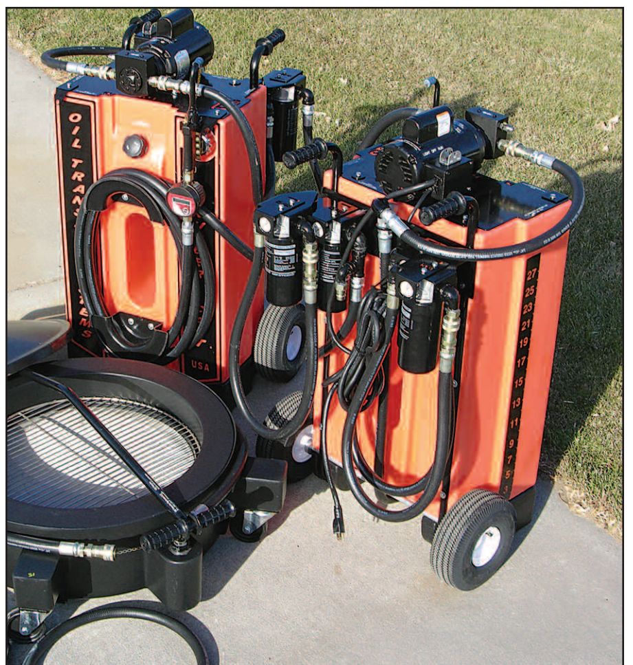
Oil Transfer Systems units are mobile and lightweight, each unit offering two sets of filters; one set can be used for new crankcase oil and the other for hydraulic fluid.
